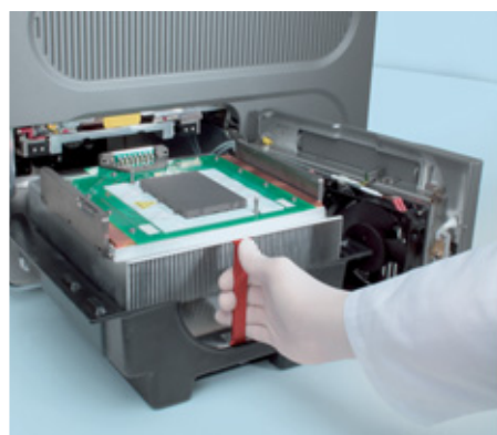
▲ Figure 1: Flexibility of the LightCycler® 480 block cycler unit. The LightCycler® 480 block cycler units (96-well/384-well format) are easily interchangeable by the user, taking no longer than a few minutes. The exchanged block cycler unit is automatically detected and identified by the system, and experiments can be pursued without time-consuming recalibration runs.
