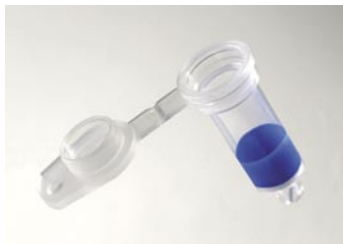
▲ Figure 1: High Pure Micro Spin Column for > 10 µl elution volume.
