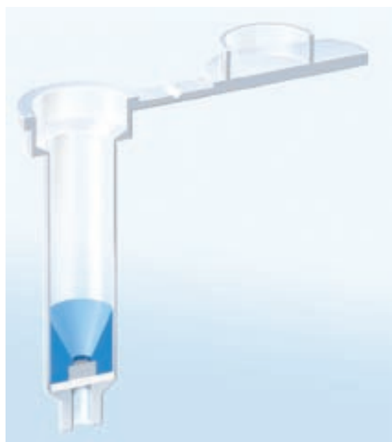
Figure 1: Cross-section view. A reducing device, designed as collecting funnel, creates a cavity for the silica membrane at the bottom of the spin column with a binding capacity of 20 \mu g. The special design of the blue colored reducing device allows easy central loading of sample and buffer up to 500 \mu l. Due to the funnel-like design, carry-over contamination is avoided. A foot-hold membrane prevents the silica membrane slipping through the outlet.
